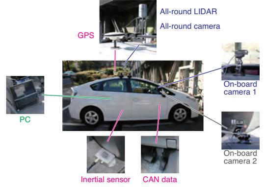
Fig. 5. Vehicle and the installed sensors used in the experiment
